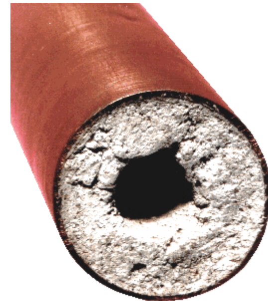
Close-up picture of hard water deposits in copper water pipes.
